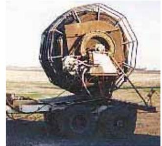
Reel mounts on an old cement mixer truck and is pto-driven through the truck's mixer drive assembly. A tractor pto drives the truck's transmission.
