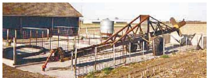
Kohnen's 43-ft. long agitator has a 6-ft. dia., four-blade propeller and mounts on the wheels off a Gleaner A2 combine.
