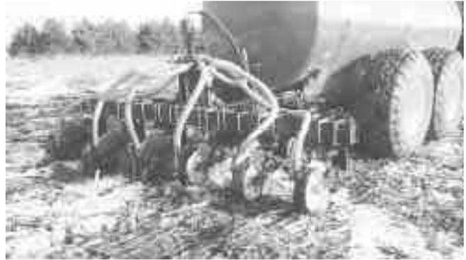
New injector system removes less than 5 percent of cover, even when working in soybean stubble.
