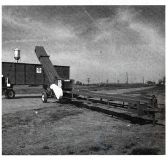
A water applicator is standard on the Crose portable baled hay slicer. Molasses applicator and pump are optional.
