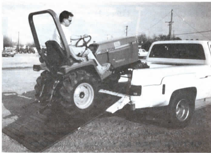
Ramp handles loads over 2,000 lbs. yet folds up to narrow 4-in. width inside tailgate.
