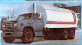
Hydraulically-controlled lids come together at the top to form rain-tight seal. In addition to grain, this first-of-its kind truck box can also be used to haul livestock or silage.
