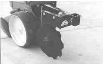
Notched blade cuts through residue as smooth blade makes trench for fertilizer.
