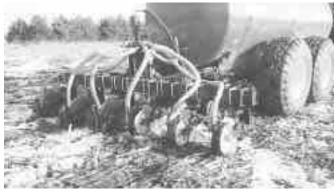
New injector system removes less than 5 percent of cover, even when working in soybean stubble.
