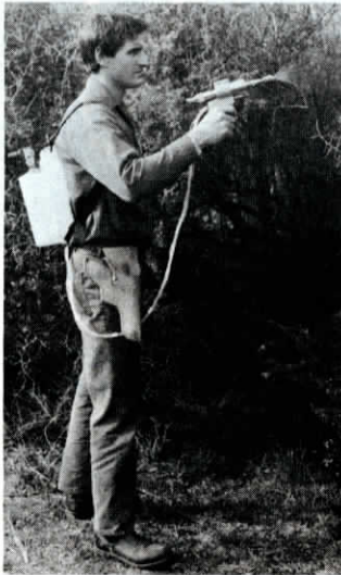
LP-gas to power spray gun can be carried in backpack for specialty spray jobs.
