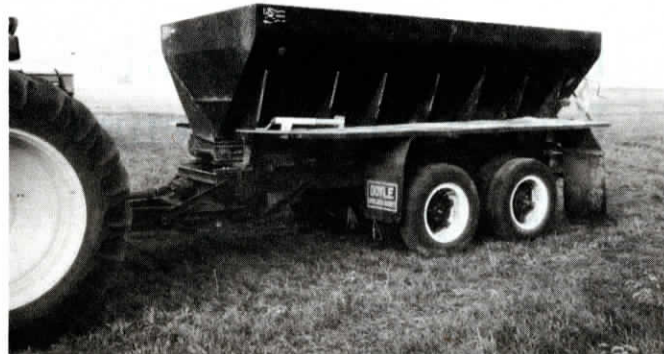
Lee Williams turns "junked" truck-mounted spreaders into tractor-pulled trailer spreaders.
