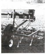
gauge wheels. Dickerson mounted the hopper's ground drive wheel on top of one gauge wheel and used a pair of chains to drive the hopper's hex shaft. "The gauge wheels weren't builtstrong enough to support the added weight of the hopper. I removed the remaining gauge wheel and use the 3-pt. to keep the cultivator at the right depth," says Dickerson.
