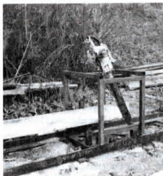
Chainsaw fitted with 32-in. bar rigid-mounts on sawmill frame. Frame rolls down track to saw log which remains stationary.
