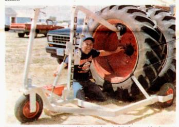
The tractor wheel spins on the small wheel at the end of the boom making it easy to line up lug bolt holes.
