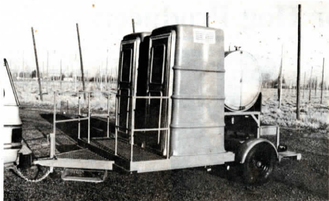
Mobile unit contains two toilets, sink, towel and soap dispensers, and a 300-gal. fresh water tank.
