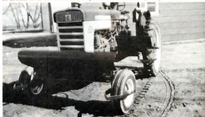
"Belly pan" on underside of tractor pushes crop down and out of the way.
