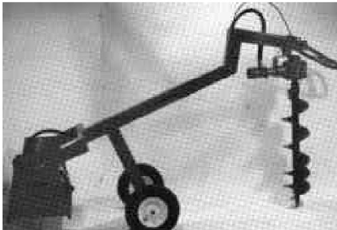
Gearbox on new digger provides 9,660 lbs. of torque, three times more than conventional direct-drive hydraulic augers.
