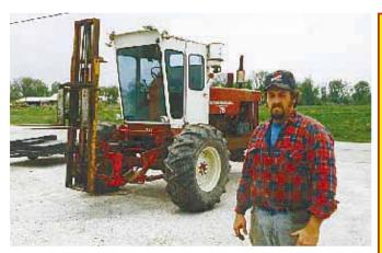
David Buss turned an IH 715 combine into a forklift by mounting a mast where the original feederhouse used to be.
