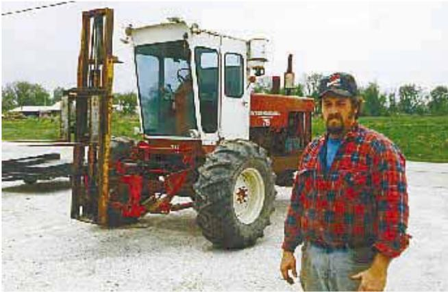
David Buss turned an IH 715 combine into a forklift by mounting a mast where the original feederhouse used to be.
