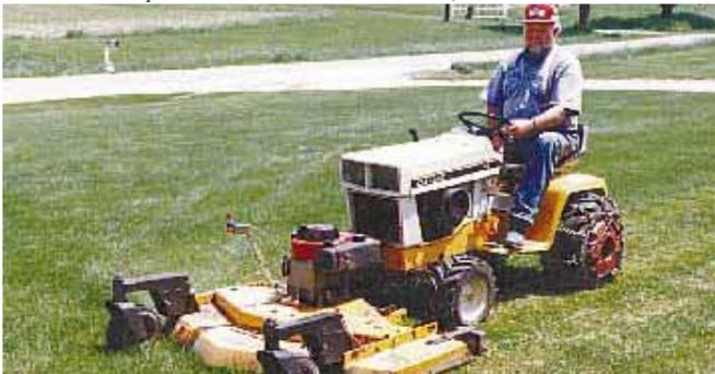
Roland Schild pushes a self-powered 48-in. deck ahead of his Cub Cadet riding mower. The new deck replaces the mower's original 36-in. deck which had worn out.
