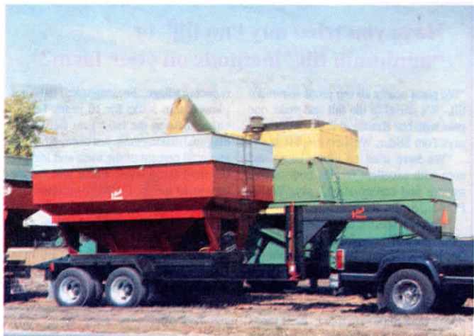
With flatbed removed, 450-bu. grain box slides onto frame of gooseneck "combo".
