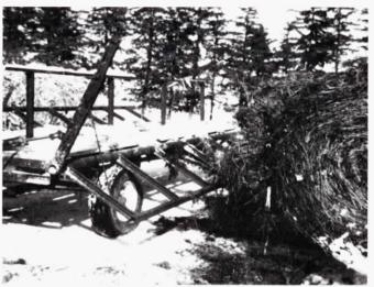
Low-cost "custom cradle" handles eight bales at a time and unloads hydraulically.
