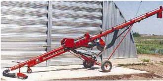
A Crary fan mounts halfway up auger to create suction to pull as much as 800 bu. per hour into modified auger.
