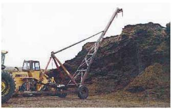
Giant hydraulically-operated hook reaches up to pull down silage from huge piles, some of which are 30 ft. high. Hook was built from an old culvert-laying machine.
