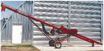
A second auger tube mounts above bottom half of original 34-ft. long auger. When you get to bottom of bin, you pull out auger stub and insert suction nozzle.
