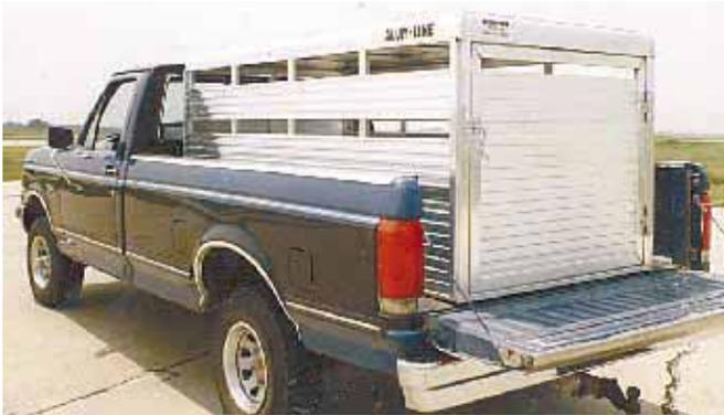
Container fits in pickup bed between the fender wells and has a full-swing endgate on back. Eliminates the hassle of using a gooseneck trailer.
