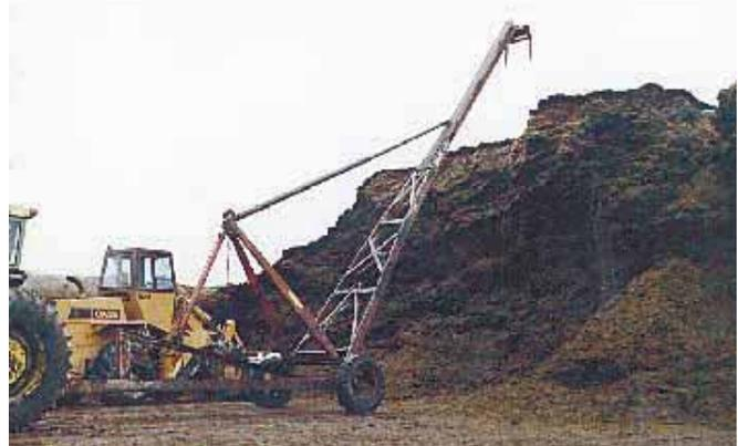
Giant hydraulically-operated hook reaches up to pull down silage from huge piles, some of which are 30 ft. high. Hook was built from an old culvert-laying machine.
