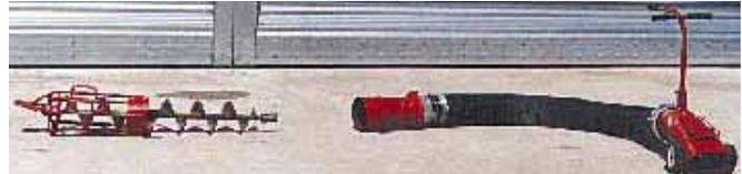
Stub auger (left) or 6-ft. flex nozzle inserts into end of auger.
