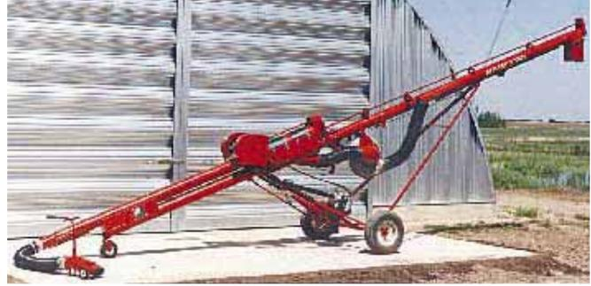
A Crary fan mounts halfway up auger to create suction to pull as much as 800 bu. per hour into modified auger.
