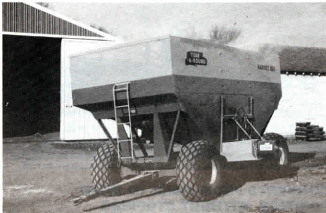
Sliding dump gate on wagon floor was replaced with new gate made from a hammermill screen.
