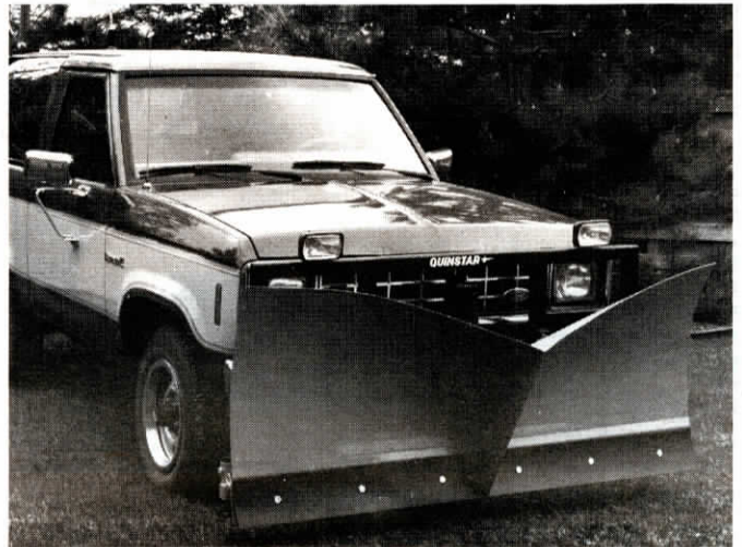
Width of original pass through snow can be widened by taking a “half bite” on subsequent passes.
