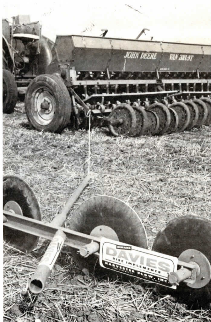
Slant of disks causes marker to want to veer sharply to left, keeping rope tight at all times.
