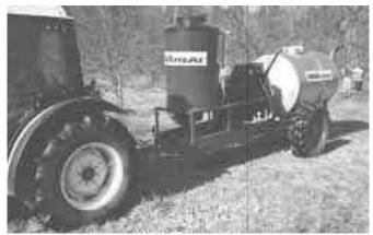
Diesel-powered machine heats water up to 220° to kill weeds. New design cuts water useage to 15 gal. per minute.
