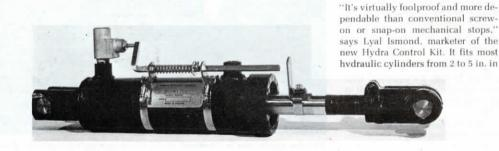
dia. with an 8 to 16 in. stroke. Optional push rods are available for shorter or longer cylinders.
