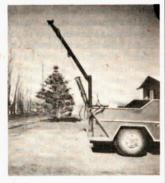
off smooth and attached two lifting loops. A 4-in. dia., 24-in. stroke hydraulic cylinder provides the lift raising the boom from its low point of 43 in. off the ground to it's high point at 11 ft., 8 in. Hydraulic power is provided by a 12-volt power pack that mounts in the corner of the box and is only activated when needed.
