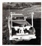
Operator controls spikes which, when released, grab bale in center and lift it into pickup.
