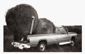
Bale mover's arms are rigid, set at width of whatever size bales are being moved. Takes only about 15 sec. to engage and load a bale.
