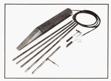
Gator Saver comes complete with power unit, straightening hull, pump, hose and about 20 ft. of insertion handles to reach past middle of 30 ft. sections of irrigation pipe. Alligator shape allows nose to slip into badly damaged areas and open enough room for rest of device.
