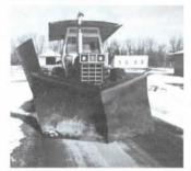
Last winter I bought this big 10-ft. wide "V" snowplow at a county auction sale for \$80 and mounted it on my 1466 IH tractor. The plow is controlled by a hydraulic cylinder on front of the tractor. It has a home-built wing on one side that's raised and lowered by a hydraulic orbit motor that drives a cable winch. Works real well around the farm. (Ernest Grotte, Rt. 1, Box 70, Finley, N. Dak. 58230 ph 701 524-2294)
