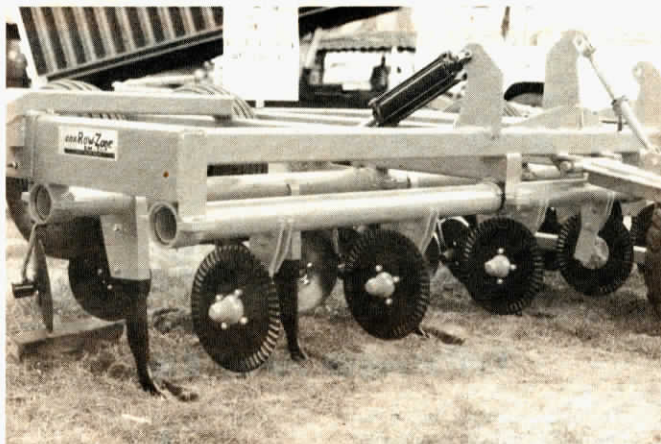
Up-front coulter which slices through trash, followed by subsoiler shanks. Disk-hillers form small ridges behind.
