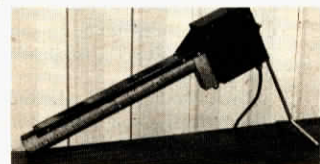
End of grain sampler auger, left, is placed in stream of grain. Samples drop into pail placed below motor, right.
