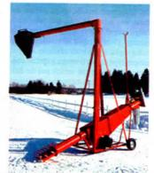
Grain cleaner blows fines through cyclone into truck or onto ground. rated tube only for com so it won't work on other grains. We aren't sure if we'll manufacture it, but if we do a 2,000 bu/hour model could probably be sold for about \$2,000, including the cyclone.
