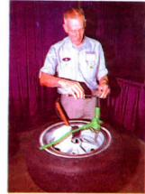
Bead breaker clamps in place over rim with insertion of small metal "key".
