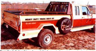
Cargo box is designed to replace existing factory-built truck boxes. Options include headache rack, side rails, notched tailgate, removable tailgate, spare tire carrier, etc.
