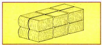
Drawing shows stacked arrangement of bales for transportation or indoor storage. For outside storage, the rounded end is positioned on top to shed water.
