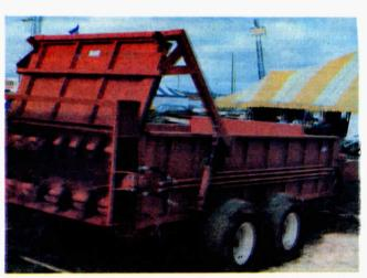
The spreader features a detachable beater assembly that can be replaced with various attachments for most any farm hauling chore.
