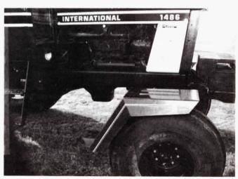
Front tire fenders provide sure footing for tractor servicing.
