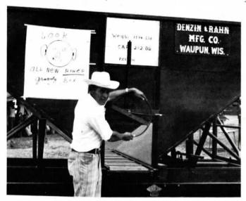
Exclusive cross conveyor and uniformly sloping sides (37°) unload ground high moisture ear corn, high moisture shelled corn and other "sticky" materials without bridging. Shown is Erwin Denzin, manufacturer.
