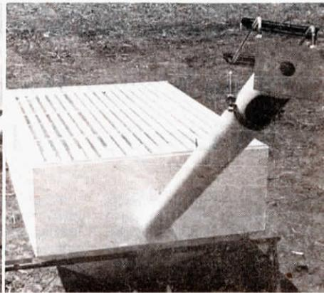
Lee Welding's 150 bu. portable unloading pit is available with or without auger. Drive-over grate will support up to 30,000 lbs., says manufacturer.
