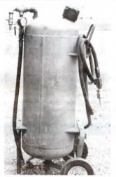
Three valves and a pressure gauge attach to the T-pipe on top of the tank. One valve is used to shut off the air supply from the compressor. Another valve regulates the amount of air in the hose coming off the "T" pipe. The third valve regulates the amount of air that goes into the tank. A valve at the bottom of the tank regulates the amount of sand that's sucked out of the tank.
