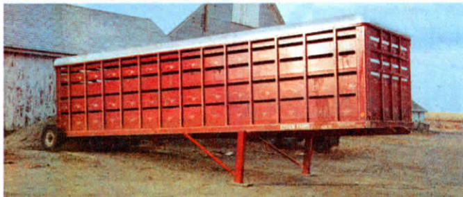
When not mounted on truck, the front end of box is held by a pair of temporary legs and a set of wheels under the back end.
