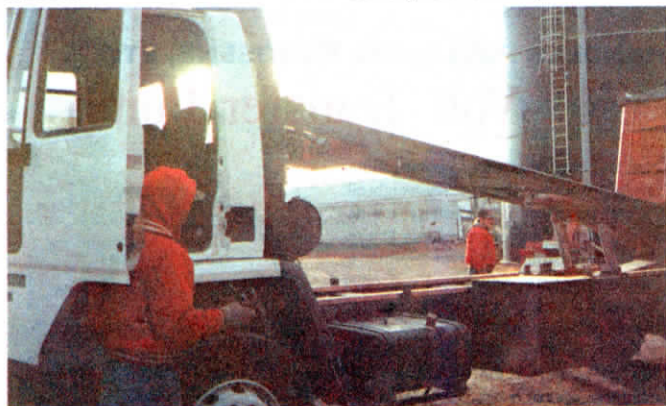
To mount the grain or livestock box, hoist raises lift rail to an incline and winch pulls it into place.
