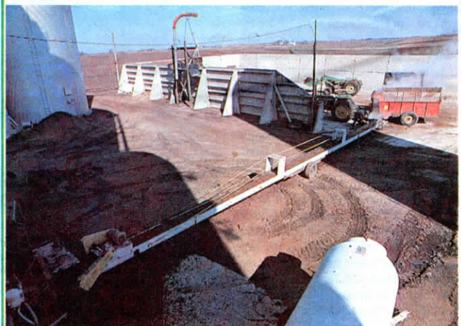
Dunn refills his vertical silos with silage from the bunker silo using a 100-ft. long rubber-belted conveyor that he loads with a front-end loader.
