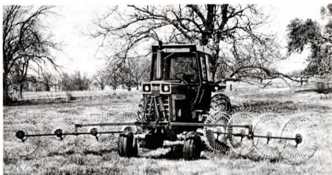
Eight-wheel rake takes 25-ft. swath and operates at speeds up to 14 mph.
