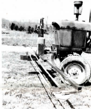
Ropes pass through chemical reservoir in center which keeps them saturated with herbicide.
