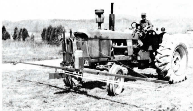
Ropes wind their way around pulleys at each end and through a set of pulleys in center.
