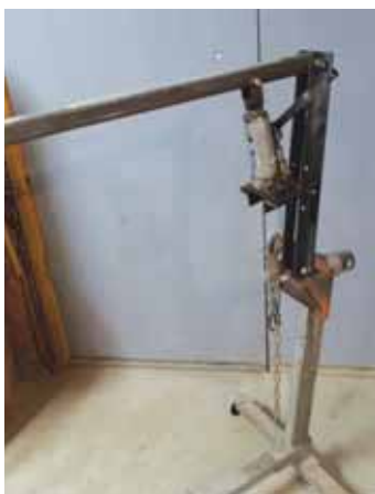
Hydraulic jack attached to the verticals provides lifting and lowering. Removing two bolts returns the engine stand to its original use.
