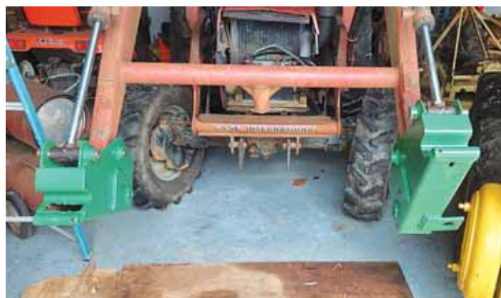
JD Quick Tach brackets installed on IH loader arms.
