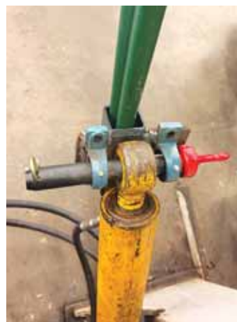
Bracket pinned to hydraulic cylinder eye.
