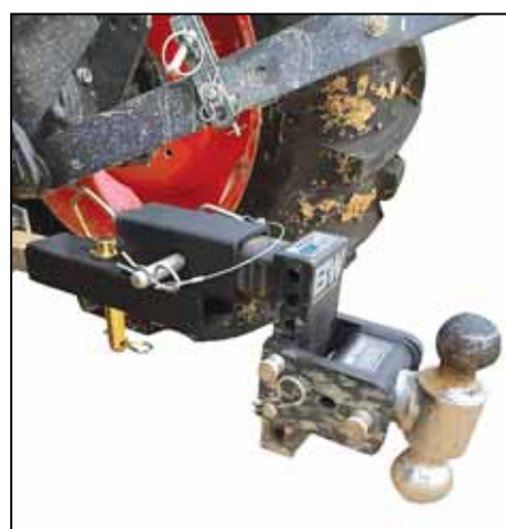
Tractor drawbar conversion kit slides over a drawbar to create a standard 2-in. receiver hitch, and no tools are required.
