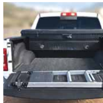
Access System kit includes a 3-step ladder, a choice of Tailgate, Cab or Crossbody Toolbox system, and mounting hardware.
