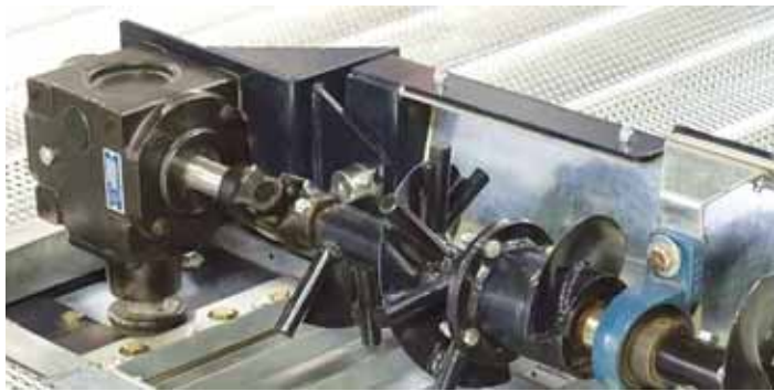
Reversing gearbox and centrifugal clutch allow it to spin freely in one direction while powering the sweep auger and the wheel in the other.
