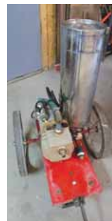
Garden waterer consists of a fire extinguisher tank mounted upside down, connected to a controller and a centrifugal pump.
