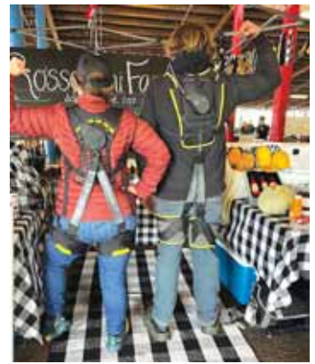
Exoskeletons are wearable suits that help support or boost what a person can normally do. They can make them stronger or improve movement.
