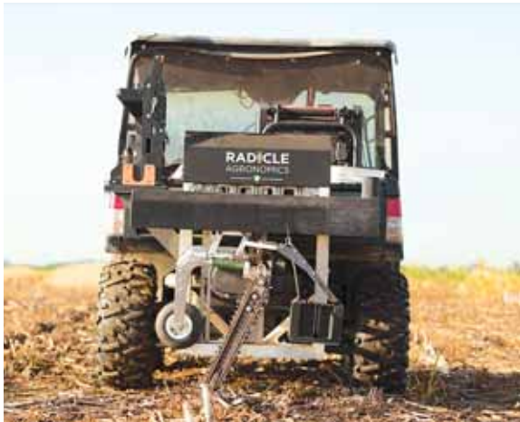
Each 30 to 40-second cycle produces roughly 6 to 8 cups of soil, representing about 40 cores.
