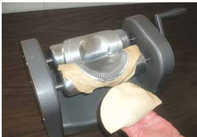
Raber's hand-cranked Fry Pie Press is a good example of their pattern-making. They originally made the patterns for the stainless-steel press and later bought the rights and inventory to market it themselves.
