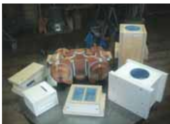
Stanley Steamer automobile cylinder block pattern and core boxes.
