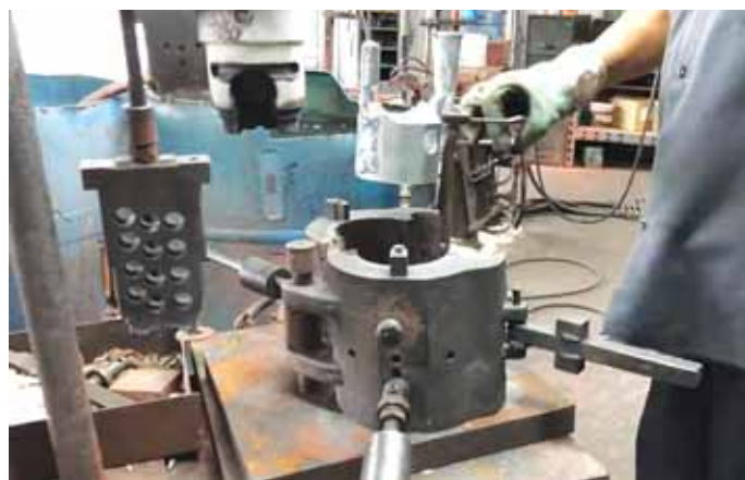
Removing molded 1964-1967 Pontiac 326 piston for machining.
