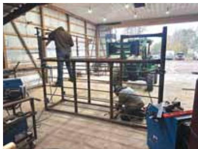
Enslinger builds a custom cattle-sorting chute on-site for a customer.
