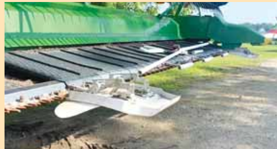
Mauck fabricated PVC deflectors by mounting a smaller pipe between Flexxifinger crop lifter brackets with a slightly larger PVC pipe on it.
