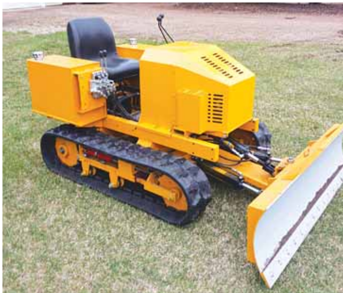
Main pump is direct-driven for the tracks, while a smaller belt-driven pump operates the nearly 5-ft wide blade.
