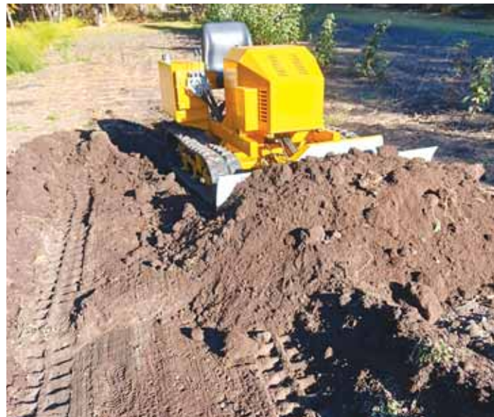
Mini dozer has rubber tracks and custom track sprockets. All components are standard off-the-shelf parts, including the 25-hp Honda engine.
