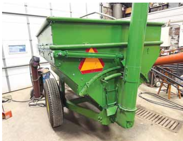
Auger lift showing hydraulic cylinder and L-bracket on outside of cart.
