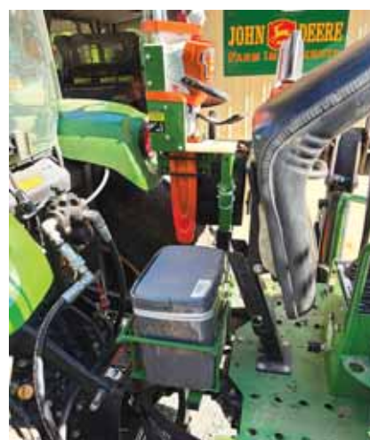
Freeman attached the frame's flat steel stock base to the 1 1/4-in. square tubing using countersunk flat head bolts, allowing the cooler to lie flat on the base.
