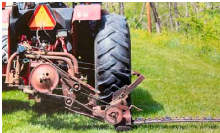
"I mounted the winch on the 3-pt. frame of the mower and made a bracket for a pulley sheave to mount on the sickle bar," says Carra.
