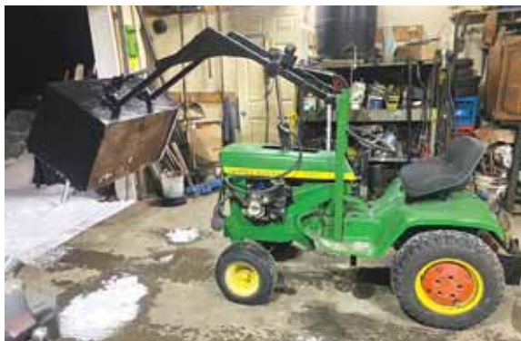
40-in. bucket was made from an old hydraulic tank Heron cut down.
