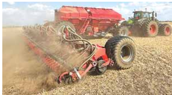
Avatar 66.10 TD combines midrow banding and single-disc seeding in a single compact unit.
