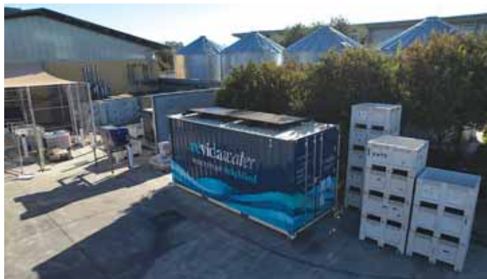
Revida's innovation lies in its containerized infrastructure. Systems arrive at farms or wineries in 20 or 40-ft containers, ready to connect to dirty and clean-water plumbing.
